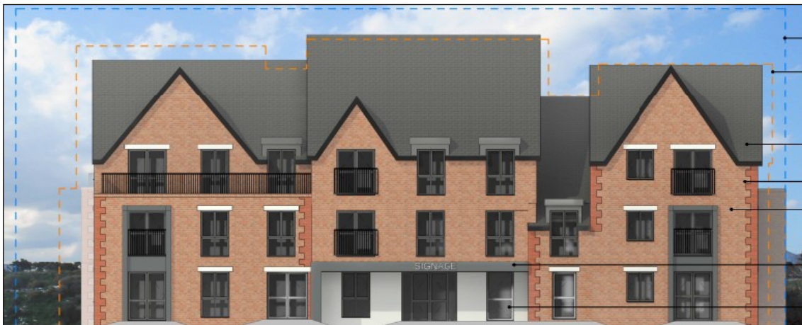
Proposed northern (Spath Road) elevation. The blue line depicts the outline of the previously refused scheme and the red line depicts the outline of the building originally proposed as part of the current application
